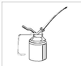
Apply refrigerant oil to the screw joints and O-rings
