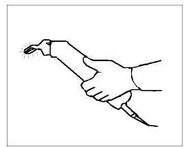
Cut using a thermocutter
