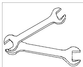
Use two spanners to evenly release or fasten refrigerant line connections
